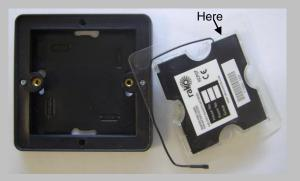
Prise rear cover from wall plate by pulling at position marked above
